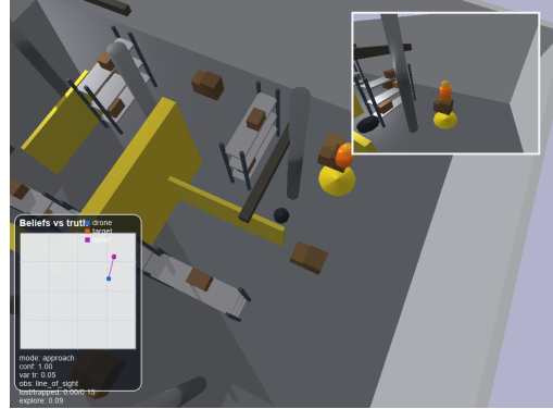
Figure 1: Compact overview of the temporally predictive scene-based drone controller. Fast local beliefs and slower scene-level beliefs are updated online, candidate actions are rolled out over a short horizon, and policy evaluation depends on both expected free energy and predicted scene improvement. Right: representative frame from the PyBullet drone simulation.
